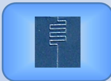
Lines drawn on FTO by laser scribing.
