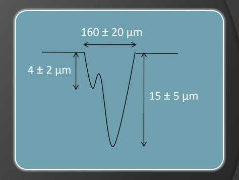
Figure shows specifications for the thinnest line we perform. We are able to carry out lines with higher thicknesses (300, 500, 1000 µm, etc.)
